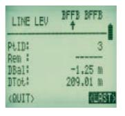
During line levelling the clear menu guidance is outstanding. Important measured and process data is displayed at once, enabling checks of measured data and on the progress made.
