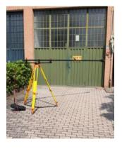
BLK WINDOWS SCAN is an easy and safe system to carry out scans in all the cases where it is necessary to arrive in inaccessible places horizontally.
